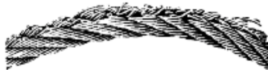
Wear caused from using a drum with an opening smaller than the ropes diameter.
